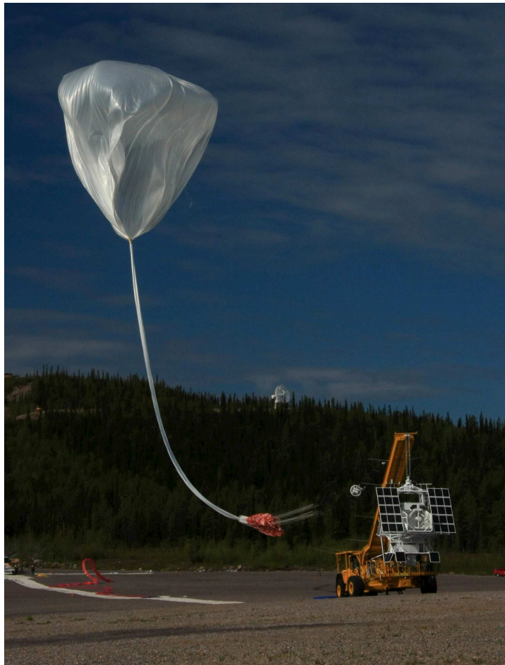
Fig. 10. The SUNRISE payload (in the foreground) just prior to launch on 8th June 2009, at ESRANGE, near Kiruna in northern Sweden. In the background, the stratospheric balloon has just been released and is slowly rising. The total weight (including the balloon and helium) is roughly 6 tons, with a payload mass of 2 tons.
